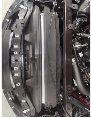
Mount the OEM radiator guard in the brackets. Then secure the radiator guard and oil cooler with included zip-ties.
