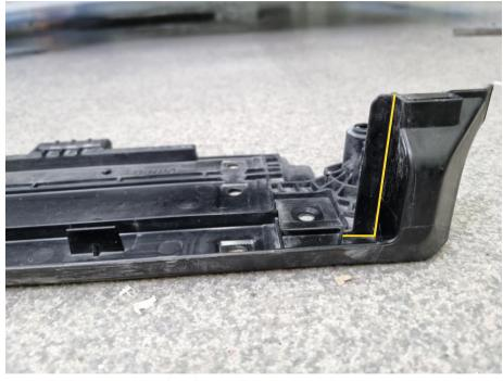
Cut the right side of the lower radiator support in a straight line down from the clip mount.
