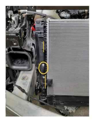
Cut the brackets according to lines in picture from the right plastic radiator support and cut the tab circled in picture flush.
