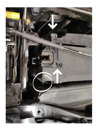
Remove the 4 x T30 screws holding the top plastic and fan to the radiator. Release the clip and lift up the fan a bit to remove the top plastic.
