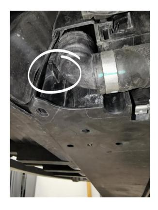
Release the clip to remove the bottom radiator connector. Then pinch the lower radiator hose and disconnect it from the radiator and drain the coolant from the radiator.
