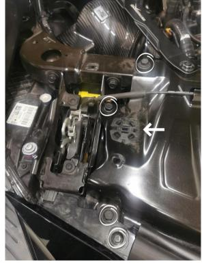
Remove the two plastic clips on each side holding the plastic panel over the hood latch.
