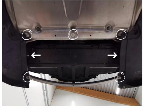
Remove the 12 x 8mm hex screws holding the bottom part of the bumper. Then preferably with the help of an assistant, remove the bumper. Start by pulling out the sides and disconnect the electrical connections on both sides, then pull the bumper forward to remove it from car.
