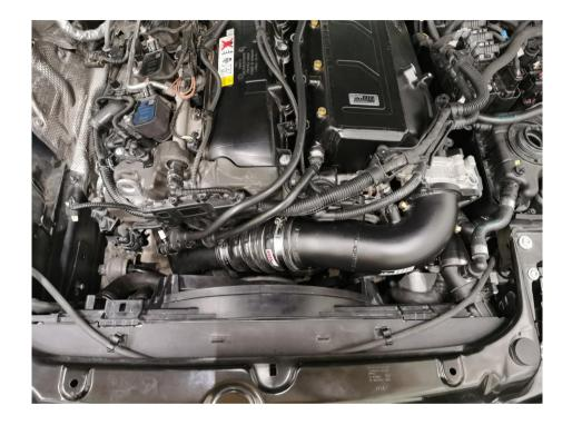
Make sure the hose sits correctly on both ends there is a little room for adjustment of angle for the turbo outlet pipe, then tighten the hose clamps to 5Nm.
