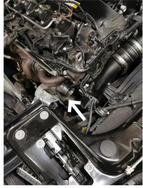
Disconnect the three electrical connections marked on picture, two in the charge pipe and one from the valvetronic motor. Now remove the  $3 \times 730$  screws holding the charge pipe to the throttle body.
