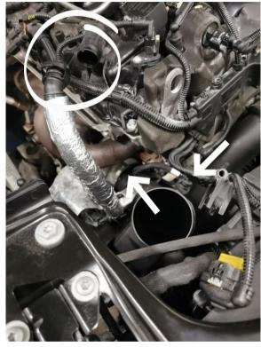
Unclip the heat protection blanket and disconnect the wastegate electrical connection underneath. Then disconnect the electrical connection in the valve cover breather hose and unclip the wires from it.
