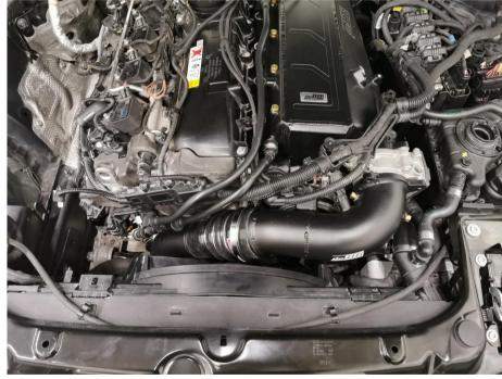
Transfer the sensors from the OEM pipe to the do88 performance pipe. Secure with included M6 Screw.
