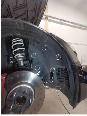
Remove the 12 x 8mm hex screws holding the bottom part of the bumper cover. Then preferably with the help of an assistant, remove the bumper. Start by pulling out the sides and disconnect the electrical connections on both sides, then pull the bumper forward to remove it from car.
