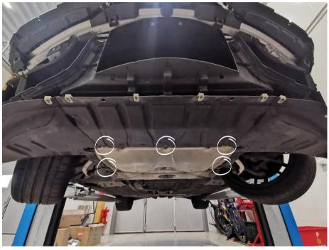
Remove the brake air duct by prying out the plastic clips and remove it in a backwards direction. Repeat on the other side.
