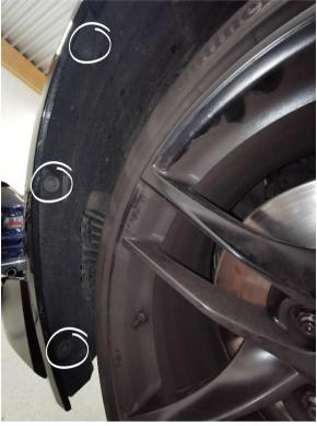
Remove the rubber seal and remove the 4 x 10mm hex screws holding the bumper cover.
