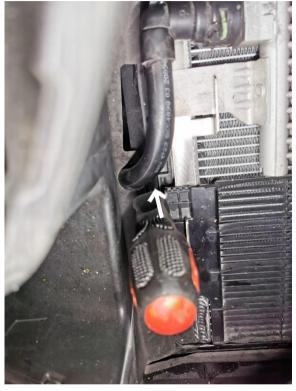
Now carefully loosen the oil line from the radiator support on both sides. Push the tab gently to release it.
