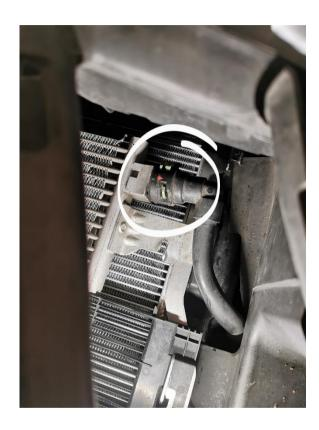
When both oil lines are separated from the radiator support, lift the oil cooler upwards and move in a forward direction to release it from its bracket.
