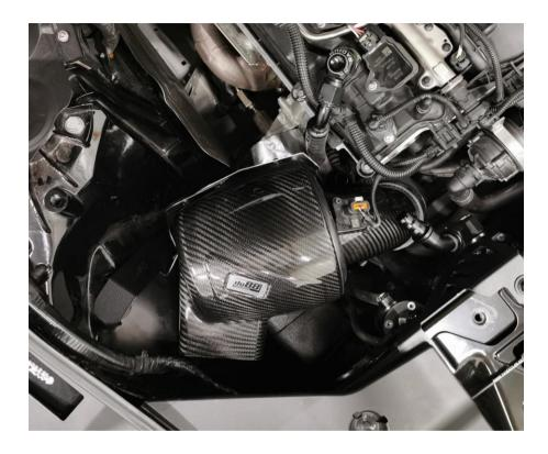
Install the filter housing assembly in the car. Start by making sure the tabs are seated correct in the OEM bushings. Then make sure the pipe is inserted far enough down the hose. Orient the hose and carbon fiber pipe together so they align well. Tighten the hose clamps to 5Nm do NOT overtighten the hose clamp on the carbon fiber pipe as it will damage it.
