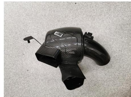
Install the do88 Performance filter and secure it with the included hose clamp, maximum fastening torque 5Nm, do NOT overtighten the hose clamp as it will damage the carbon fiber pipe.
