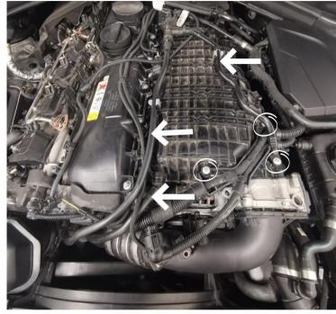
Remove the 3 T30 screws that holds the charge pipe to the throttle body.
