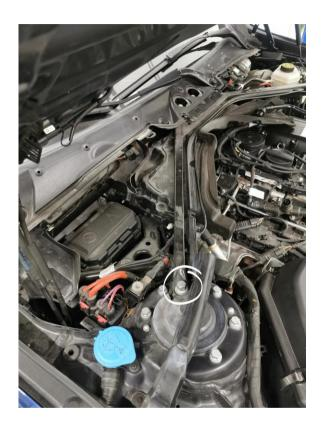
To reveal the outer strut brace mount, remove the right and left side plastic covers by twisting the 6 plastic 10mm Hex nuts in the rear and remove. Then remove the 1 x 10 mm Hex screw on each side holding strut brace to the strut tower.
