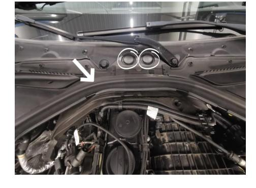
Disconnect the EVAP valve from the line coming from gas tank and place it to the side.
