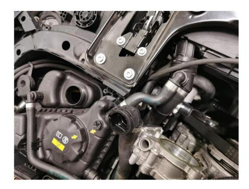
Disconnect the coolant hose going to the water pump junction and cap it of at the junction.
