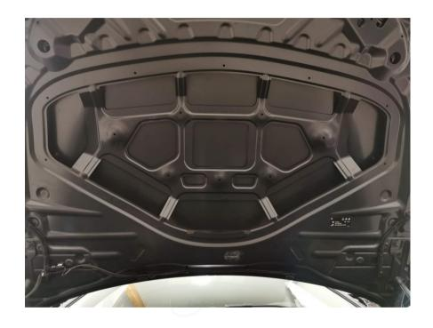
Carefully close the hood to check clearance from engine cover.
