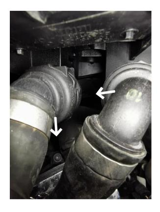
Disconnect the intake manifold water outlet and inlet.
