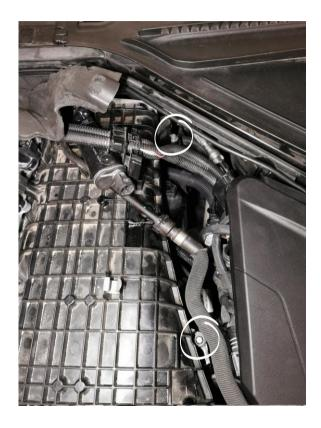
Loosen the 2 x  $\rm E10$  screws holding the intake manifold to the brackets on the left side.
