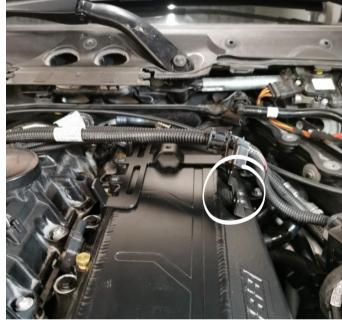
Mount the large bracket on top of the intake manifold using 3  $\times$  M5 screws included.
