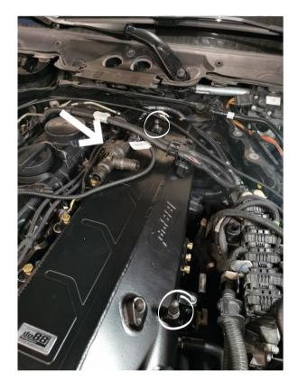
Mount the EVAP valve to the large bracket.
