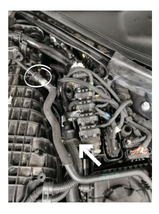
Disconnect the coolant bleeder hose from the inlet manifold and cap the inlet manifold side with the included cap.
