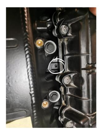
Now mount the do88 Performance intake manifold in the car the same way the OE one came out. Position manifold centered over the headless screws and back them out until they are halfway into the manifold flange.
