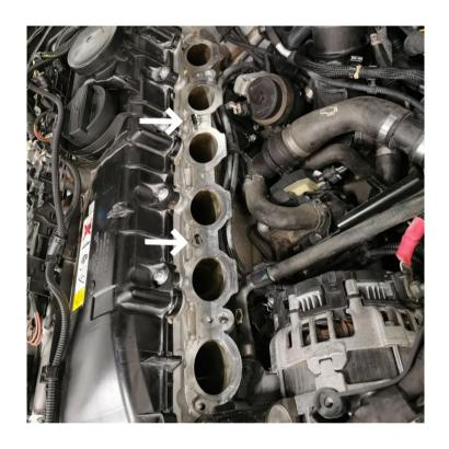
At this point make sure there are no dirt or debris in the cylinder head runners.
