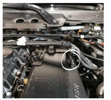
Mount the large bracket on top of the intake manifold using 3 x M5 screws included.
