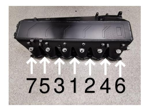
Now mount the do88 Performance intake manifold in the car the same way the OE one came out. Position manifold centered over the headless screws and back them out until they are halfway into the manifold flange.
