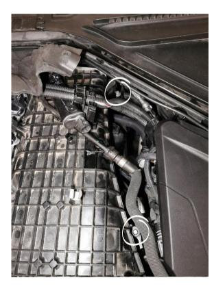
Loosen the 2 x E10 screws holding the intake manifold to the brackets on the left side.
