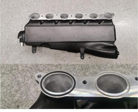
Install 6 of the included sealing rings to the Thermal barrier spacer.
