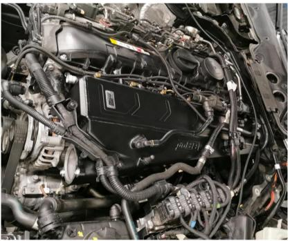
The intake tank EVAP line have to be shortened to fit. Heat the end of the EVAP line where it sits on the fitting that installs in the inlet tank of the intake manifold and pull it apart.
