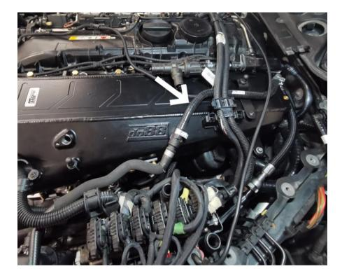
Connect the EVAP canister to the valve using the small included aluminum joiner and included fuel hose (cut the fuel hose to suitable length). Secure with hose clamps and fasten the canister to the large bracket with included zip-tie.
