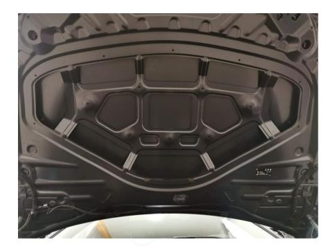
Carefully close the hood to check clearance from engine cover. You might need to remove in hood sound isolation (if present) to clear the engine cover.
