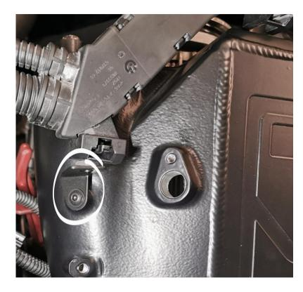
Fasten the rear bracket for the front wiring channel to the intake manifold with 1  ${\rm x}$  M5 screw included.
