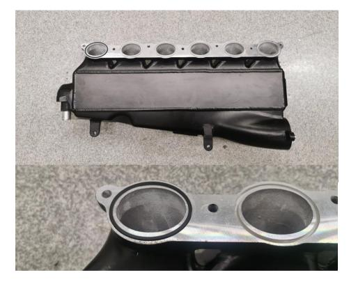
Mount 6pcs of the included sealing rings to the intake manifold flange.
