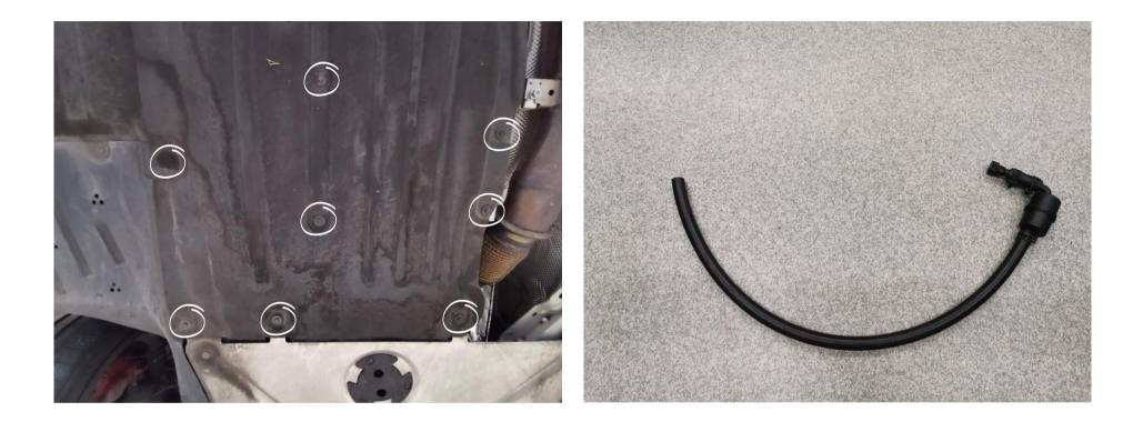
Remove 8 x 8mm hex screws from the underflooring and remove it to reveal the lower EVAP connection (the black plastic line in the transmission tunnel). Disconnect it and remove it upwards.
