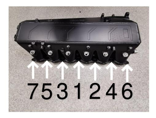
Mount the do88 Performance intake manifold to the cylinder head. Align it over the headless screws and backing them out until they are halfway into the manifold flange.
