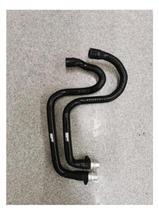
Mount the included quick connector adapters to the do88 performance silicone hoses and secure with included hose clamps (torque to 5Nm).
