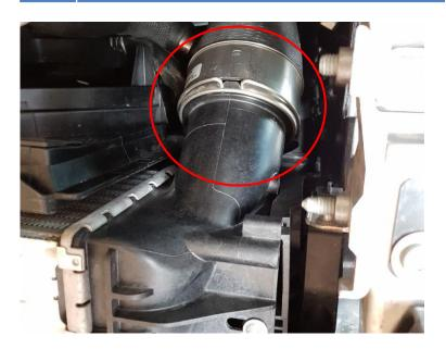
Pry the plastic tabs free on both sides for the front intercooler air guide.
