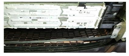
4. Remove 1x Torx T27 on each side of the intercooler then gently remove the intercooler from the car.
